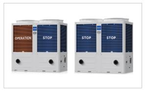
In combination system the defrosting of one of module does not affect the other modules operation. If one unit is defrosting the other heat units, naintaining heating operation this realises non-stop system heating during defrosting.
