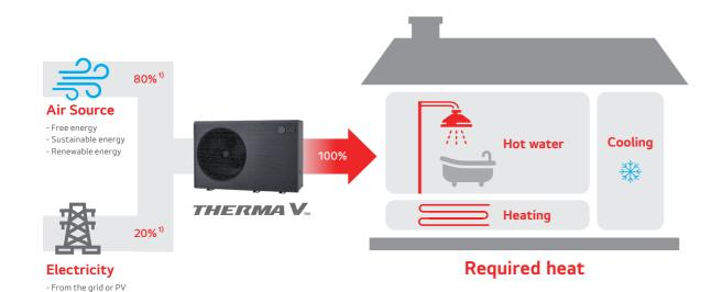
1) The efficiency ratio is to help general understanding and is based on the Seasonal Coefficient of Performance (SCOP) of THERMA V R290 Monobloc under Low Temperature & Average Climate conditions, which is higher than 5. The actual efficiency may vary with water and outside temperatures.
