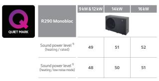
1) Sound power level is measured in accordance with EN 12102-1 and ISO 9614.
