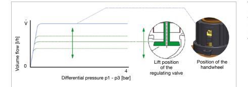
The **integrated diaphragm** unit (pos. 1a) keeps the differential pressure "p1"-"p2" at a constant level via the regulating unit (pos. 2) which is activated through the actuator and via the nominal value unit (pos. 1b) which can be set to a maximum flow value. Even where high differential pressure variations "p1" - "p3" occur, e.g. if sections of the system are activated or inactivated, the differential pressure "p1" - "p2" is kept at a constant level.
