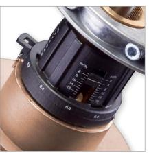
The nominal values are imprinted on three peripheral scales ensuring an excellent optical display of the values in any installation position. The nominal values can be set in m<sup>3</sup>/h. The locking clip can be lead sealed to secure the setting from unauthorized access.
