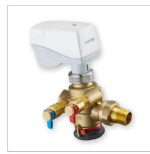
"Cocon QTZ" with electromotive actuator for modulating control (0-10V) with connection thread M 30 x 1.5. Function and characteristic line selection via a DIP switch. For use in central heating and cooling systems for precise flow and temperature control.
