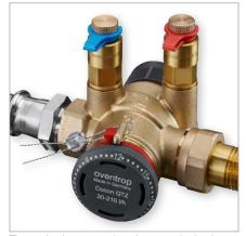
The setting is protected against unauthorised tampering with the help of the handwheel which engages automatically. The setting can be additionally secured by inserting the red locking ring which can be lead sealed. Even with the actuator in place, the settings of the "Cocon QTZ" can be read off and adjusted.
