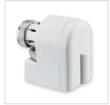
Electromotive actuator with connection thread M 30 x 1.5. For room temperature control in conjunction with two point controllers. For use in radiant and chilled ceiling systems as well as induction air systems.
