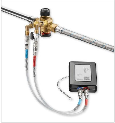
The pump setting can be optimised with the help of a measuring gauge, such as the "OV-DMC 3". For this purpose the pump head is reduced until the "Cocon QTZ" is just working within the control range.
