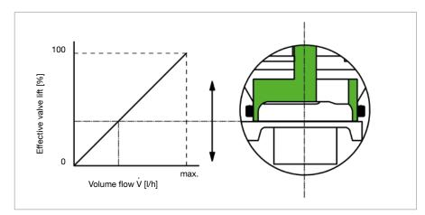
The **integrated diaphragm unit** (pos. 1a) keeps the differential pressure "p1"-"p2" at a constant level via the regulating unit (pos. 2) which is activated through the actuator and via the nominal value unit (pos. 1b) which can be set to a maximum flow value.
