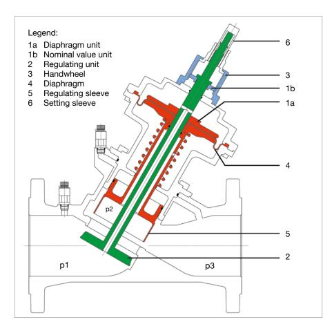
The required **flow rate** is set with the help of the handwheel (pos. 3). The illustrated section shows three pressure ranges: "p1" is the inlet and "p3" the outlet pressure of the valve. "p2" is the pressure actuating the diaphragm unit (pos. 1a) which keeps the differential pressure "p1"-"p2" at a constant level.
