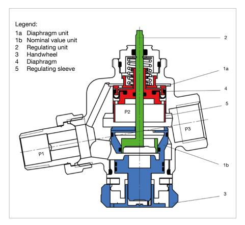
The required **flow rate** is set with the help of the handwheel (pos. 3). The illustrated section shows three pressure ranges: "p1" is the inlet and "p3" the outlet pressure of the valve. "p2" is the pressure actuating the diaphragm unit (pos. 1a) which keeps the differential pressure "p1"-"p2" at a constant level.
