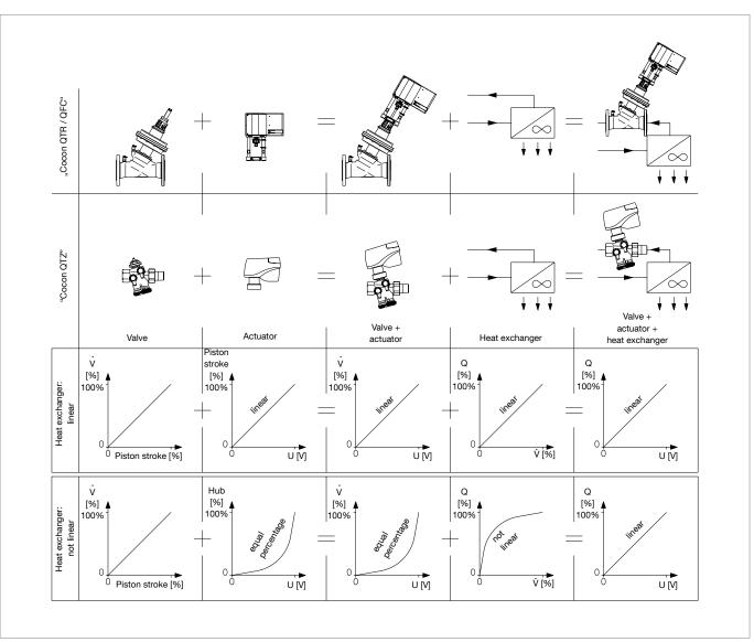
Optimisation of the interaction of valve, actuator and heat exchanger with modulating 0-10 V actuators. The illustration shows idealised characteristic lines explaining the control principle.
