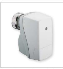
Electromotive actuator with connection thread M 30 x 1.5. For room temperature control in conjunction with three point controllers. For use in radiant and chilled ceiling systems as well as induction air systems.
