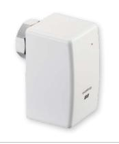
Electromotive actuator with connection thread M  $30 \times 1.5$ , system EIB, with integrated bus coupling. The electromotive actuator EIB is suitable for the direct connection to the European installation bus control system. The power absorption is extremely low, so that a separate power supply is not needed.
