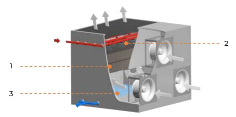
The hot water to be cooled is pumped to the top of the cooler through a pipe and then distributed over the heat exchange surface (1) by distribution nozzles (2).
