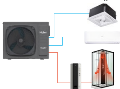
Scenario 5: Domestic Hot Water + AC Cooling
